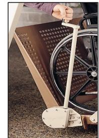
Standard Adult or Child-size wheelchairs: The back of the large wheels should extend three to four inches behind the edge of the platform.
